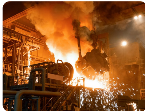
Figure 17: Ladle Metallurgy Furnace (Getty Images)
