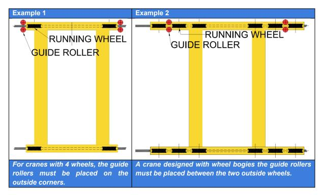
The design of the guide rollers must meet the following requirements:
