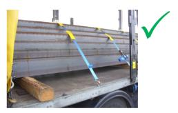
It is important to note that each strap used to keep the product on the trailer works as part of a system of restraints where failure of one component could compromise the entire system.
