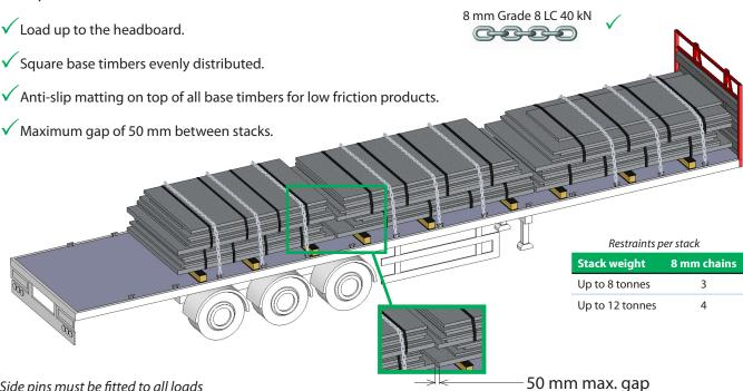
Side pins must be fitted to all loads
