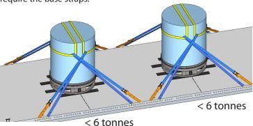
**DO NOT** put hooks on spring lashings - they will damage the coil.
