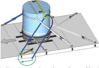
Lashing point #1 must be past the outer diameter of the coil.
