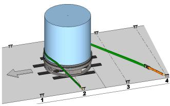
Lashing point #2 must not be in front of centre of the coil.
