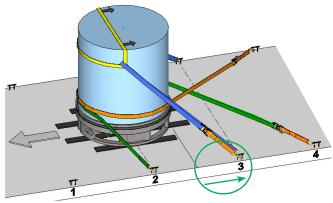
Lashing point #3 must be past the outer diameter of the coil.
