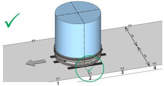
Centre of the coil in line with the lashing point #2 or just in front:
