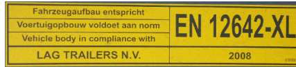
Typical plaque on a trailer with a headboard rated to EN 12642 Code XL.
